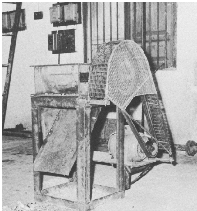
FIG. 1. Mango stone decorticator—front view showing the complete setup.
